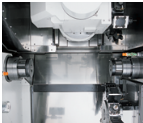
Simultaneous upper & lower right side cutting
