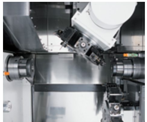
Simultaneous upper & lower right side milling
